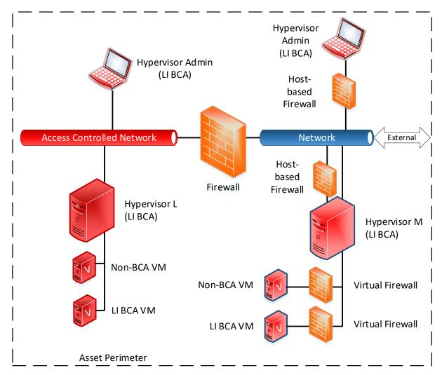
In the example illustrated above, the virtualized infrastructure supports BES Cyber Systems that are at a low impact level. Two hypervisors are shown each with a different method used to permit only necessary inbound and outbound electronic access to the hypervisor and its VMs.
